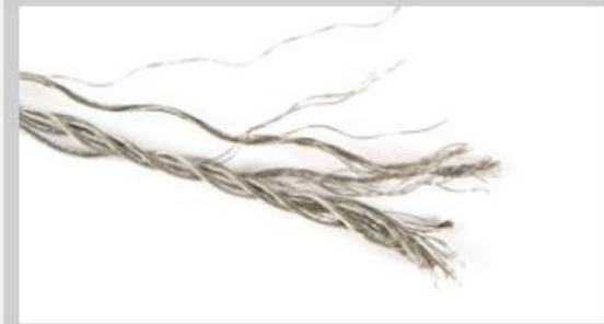
Traditional cable lifeline (with energy absorber) failure
