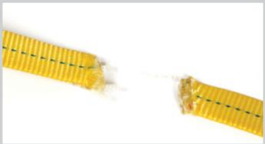
Traditional webbing lifeline (with energy absorber) failure
